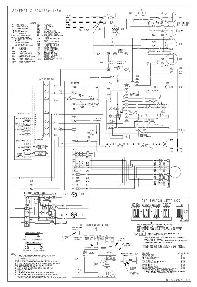
Fig. 15—ICM FIOP Electric Schematic—Unit 48JZ
